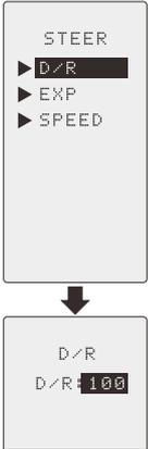
Adjust the positive and negative travel of steering channel simply .
