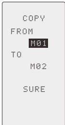
Copy the currently selected model data to another , without changing the current model data . You can simply set parameters of models that only has few difference by this function .
