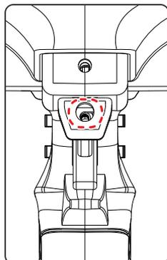
Trigger tension adjusting screw
