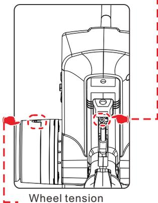
Wheel tension adjusting screw
