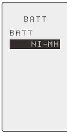
Different battery needs to select different power supply scheme. If not choose properly, it will not damage the transmitter. But it will affect the life of the battery.
