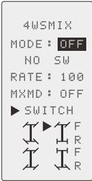
The action of the steering channel through the mixing control make the CH3 control the movement of back wheel .
