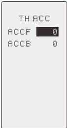
Adjust operation amount near the throttle acceleration and brake neutral position .
